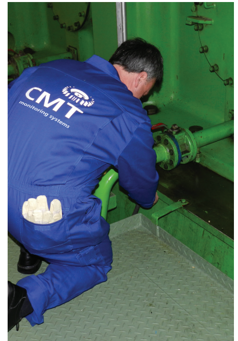
Taking a cylinder drain oil sample from the scavenge space.
